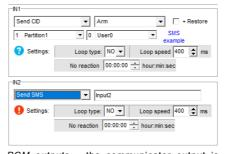
PGM outputs - the communicator output is programmed in this settings window. The control command to be entered when sending an SMS depends on the selected PGM output function:
